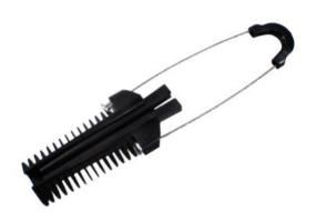
Telenco® AC35L clamps are used for the dead-ending of aerial figure-8 cables with FRP or steel messenger on access networks where spans do not exceed 90 meters.
